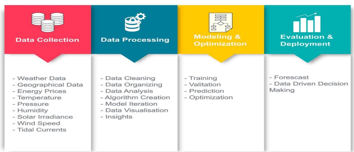
Figure 2: Hassan et al. Data Preprocessing Pipeline for Renewable Energy Data
